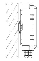
• DIN-rail mounting by using PCB bracket
