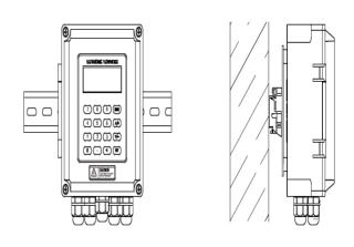
Converter of ISE-2000B can be installed on the wall or in distribution box and explosionproof box
