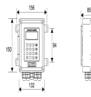
Wall mounting: Fix the converter with 4 Φ6 expansion bolts or normal nails.
